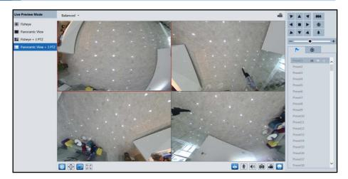
**4PTZ view mode** (you need to switch the stream mode in the fisheye parameter interface)
