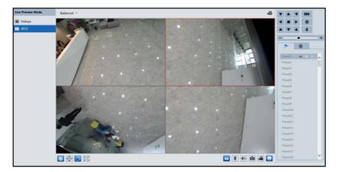
In panoramic + 3PTZ view mode or fisheye + 3PTZ view mode or 4PTZ view mode, select a PTZ window and view the image from every direction by controlling PTZ panel.
