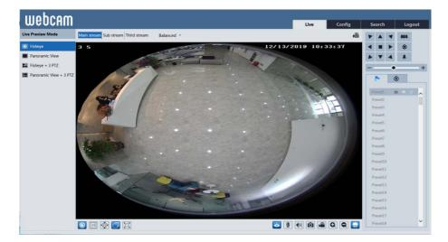
In the live mode, the different streams and live view modes can be switched as needed. The following table is the instructions of the icons on the live view interface.
