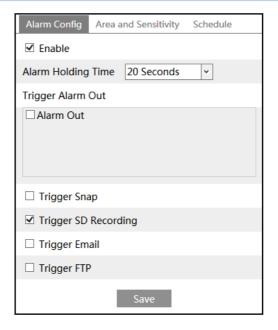
1. Check "Enable" check box to activate motion based alarms. If unchecked, the camera will not send out any signals to trigger motion-based recording to the NVR or CMS, even if there is motion in the video.
